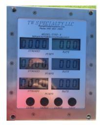
Model 5700-3 monitors up to 3 pumps and displays total strokes and rate per minute for the pump. The test button will test the unit @ 60 SPM. Zero buttons are used to zero total strokes.
